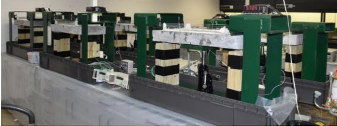
Figure 11 Typical Setup of Accelerated Corrosion Tests
