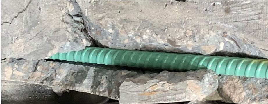
Figure 29 Lack of Bond Between Epoxy-Coated Bars and Concrete Under Static Loading
